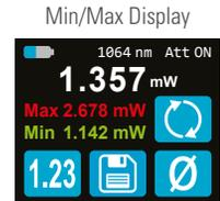
In addition to the Real Time value, the device displays the lowest and highest values
