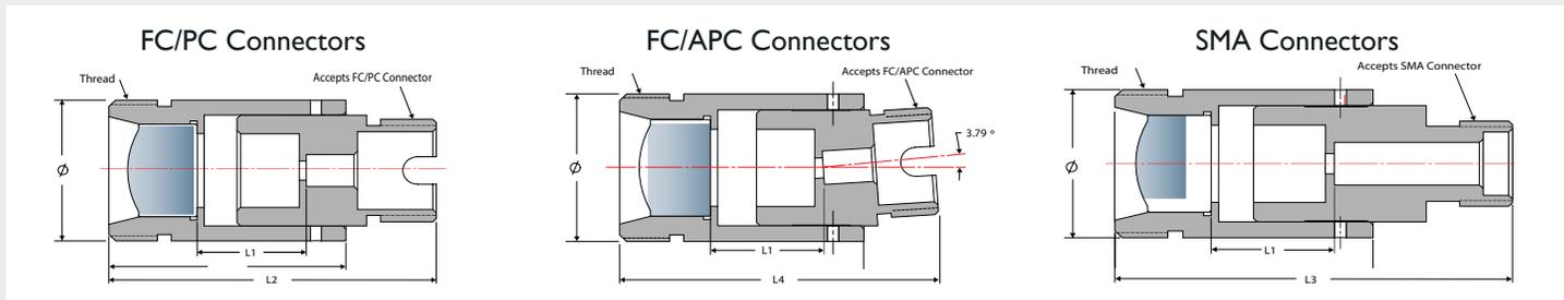
For all Connectorized Collimators, Pointing Accuracy =  $0.5^\circ$  and Waist Position = Infinity
