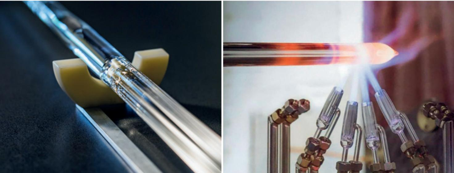
As one of the few suppliers on the market, CeramOptec® covers the entire manufacturing chain from the preform to the assembled fiber bundle. The preform sets both the optical properties as well as the geometry of the glass fiber drawn from it. Our in-house production gives us full control over these important parameters and enables us to adapt them quickly and flexibly to your requirements.
