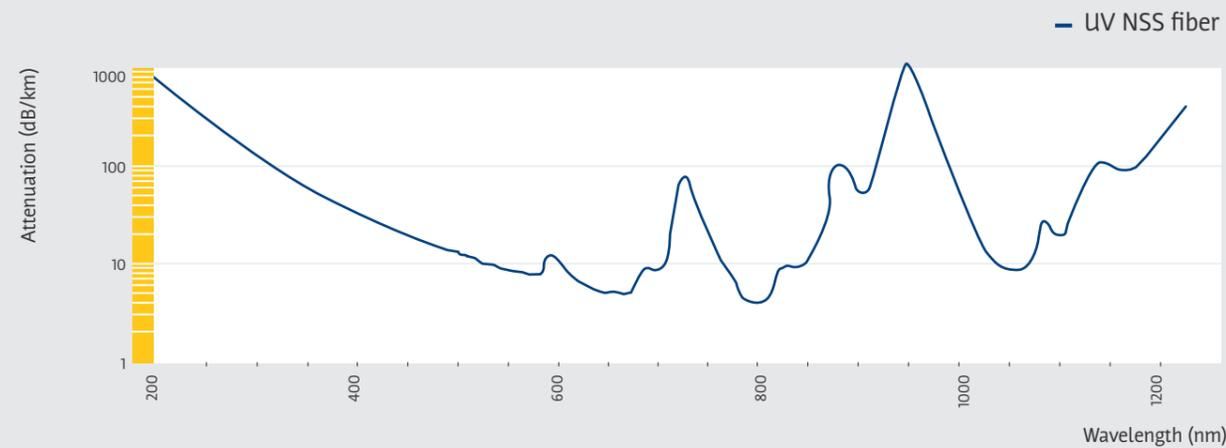
Optran® UV NSS (Comparison of solarization resistance)
