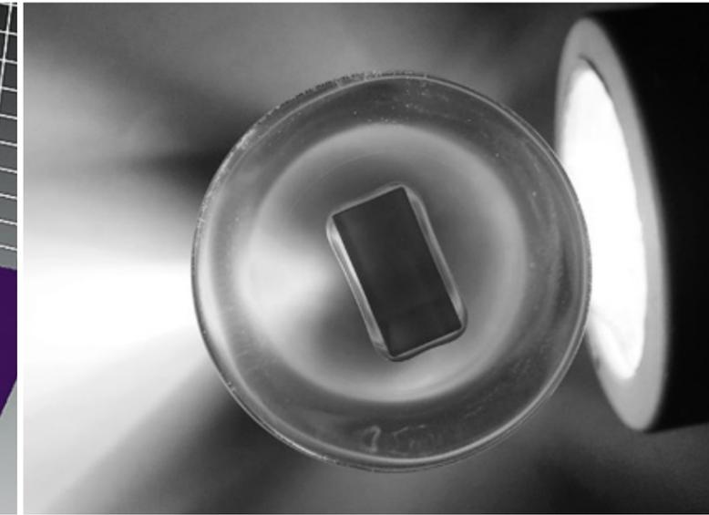
Fibers with a rectangular core geometry homogenize the intensity distribution. The image shows the intensity distribution on the focal level, using NCC fibers with core diameter of 800 × 800 μm.
