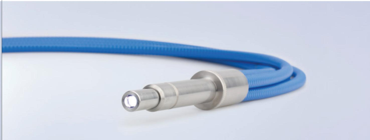
CeramOptec®'s fused-end PowerLightGuide bundles set the benchmark for consistently high long-term performance. The fusing process completely eliminates inter-fiber spaces and thus positions CeramOptec®'s PowerLightGuide bundles among the most sophisticated fiber bundles on the market. As the bundles do not rely on adhesive, they are resistant to temperatures of more than +600 °C, making them the first choice for demanding applications!
