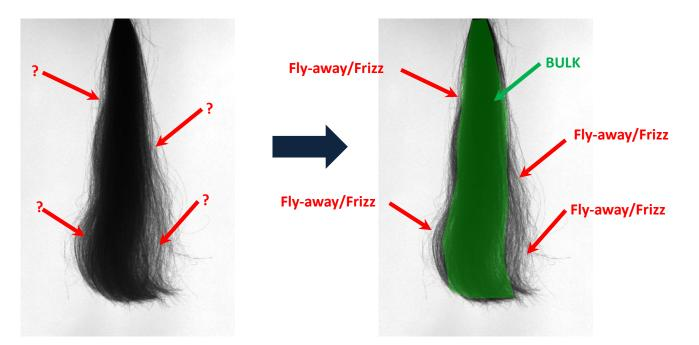
Need for image processing to determine boundaries and determine BULK and FLY-AWAY/FRIZZ.
