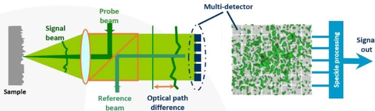
Each homodyne signal is processed in parallel using a patented signal processing architecture, based on "random quadrature" demodulation scheme taking advantage of the random phase distribution inherent to speckle light. The detectors produce a time-varying analog voltage that is proportional to the rectified instantaneous surface displacement at ultrasonic frequencies.
