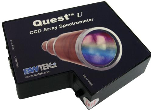
The Quest™ U is a linear CCD array spectrometer optimized for UV performance using a low stray light optical bench. It features a 2048 element detector, built-in 16-bit digitizer, USB 2.0 interface with a >2.0 MHz readout speed, and external trigger. The Quest™ U is temperature compensated, which greatly reduces the thermal drift to ~15 counts/°C. This gives improved stability by decreasing baseline drift and sustaining the dynamic range.
