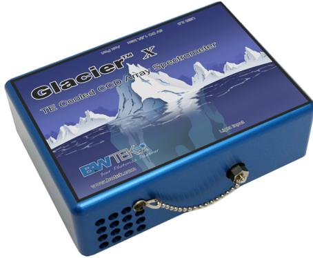
The Glacier® X is a TE cooled linear CCD array spectrometer. It features a 2048 element detector, built-in 16-bit digitizer, and USB 2.0 interface. Compared to non-cooled CCD spectrometers, the Glacier X offers higher dynamic range, significantly reduced dark counts, and superior long-term operation stability, making it ideal for low light level detection and long-term monitoring applications.
