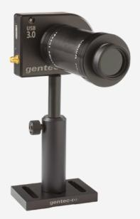
Typically, a CMOS silicon sensor is operating at its full potential when imaging lasers with wavelengths between 350 nm and 1150 nm. If you want to extend the performance range of your Beamage beam profiling camera to the near-IR telecom wavelengths band, you can use the IR Adaptor. This ideal solution takes advantage of a multi-photon absorption process to extend the sensitivity range of the camera sensor to a portion of the near-IR spectrum (1495 nm - 1595 nm).
