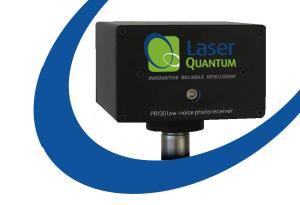
PR130 is a multi-purpose low-noise photoreceiver intended to detect a small AC signal on a large DC component. It is ideally suited for highly sensitive optical signal detection at wavelengths between 320nm and 1000nm.
