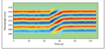
Out-of-loop measured interference of  $10^{11}$  oscillator pulses generated with a CEP Zero lock proving an excellent performance of this technology. The phase is tuned by inserting glass wedges in the extra-cavity beam as shown in the middle part of the picture.
