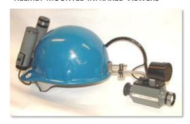
The FIND-R-SCOPE® 85050 is a self-contained, handsfree, Helmet-Mounted Infrared Viewer operating in the near-infrared region of the spectrum. A highresolution image converter tube and high voltage power supply combine with precision optics to permit a clear view of objects or images which can not otherwise be seen by the naked eye.
