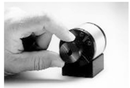
Center wavelength is adjusted by turning output polarizer.
