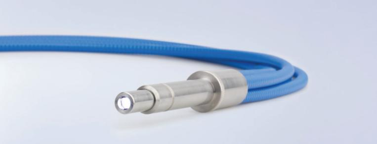
CeramOptec<sup>®</sup>'s fused-end PowerLightGuide bundles set the benchmark for consistently high long-term performance. The fusing process completely eliminates inter-fiber spaces and thus positions CeramOptec<sup>®</sup>'s PowerLightGuide bundles among the most sophisticated fiber bundles on the market. As the bundles do not rely on adhesive, they are resistant to temperatures of more than +600 °C, making them the first choice for demanding applications!
