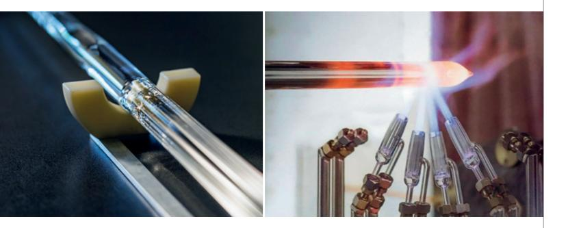
As one of the few suppliers on the market, CeramOptec<sup>®</sup> covers the entire manufacturing chain from the preform to the assembled fiber bundle. The preform sets both the optical properties as well as the geometry of the glass fiber drawn from it. Our in-house production gives us full control over these important parameters and enables us to adapt them quickly and flexibly to your requirements.
