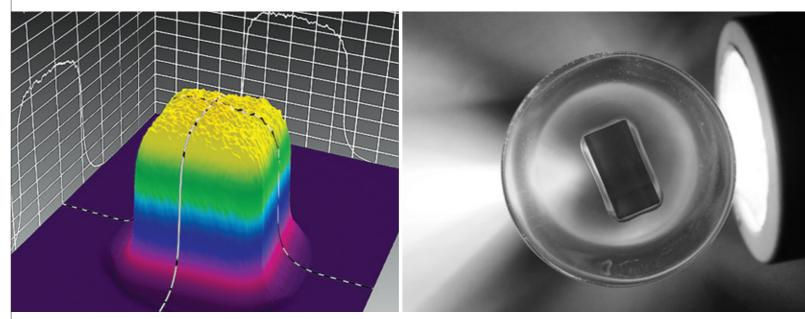
Fibers with a rectangular core geometry homogenize the intensity distribution. The image shows the intensity distribution on the focal level, using NCC fibers with core diameter of 800 × 800 µm.
