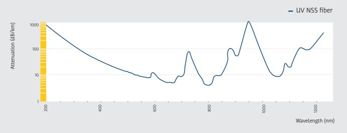
Optran<sup>®</sup> UV NSS (Comparison of solarization resistance)
