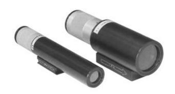
The simple telescope body enables adjustment of the spacing between the lenses for focusing, collimating or diverging. In general, we can match any combination of our BestForm Lenses to meet a very wide variety of conditions and expansion ratios from 2.5X to 50X. The Lenses are multilayer antireflection coated for peak transmittance of >96% through the pair. We will specifically fabricate custom brackets or adapters to fit the telecope to existing apparatus as required.
