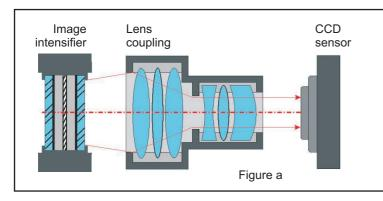
Figure a: Schematic sketch of the lens coupled intensified CCD camera. The appropriate coupling lens images the phosphor screen of the image intensifier to the CCD sensor.
