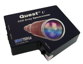
The Quest<sup>TM</sup> U is a linear CCD array spectrometer optimized for UV performance using a low stray light optical bench. It features a 2048 element detector, built-in 16-bit digitizer, USB 2.0 interface with a >2.0 MHz readout speed, and external trigger. The Quest<sup>TM</sup> U is temperature compensated, which greatly reduces the thermal drift to ~15 counts/°C. This gives improved stability by decreasing baseline drift and sustaining the dynamic range.
