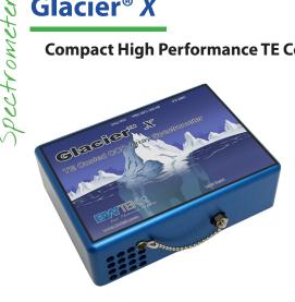
The Glacier® X is a TE cooled linear CCD array spectrometer. It features a 2048 element detector, built-in 16-bit digitizer, and USB 2.0 interface. Compared to non-cooled CCD spectrometers, the Glacier *X* offers higher dynamic range, significantly reduced dark counts, and superior long-term operation stability, making it ideal for low light level detection and long-term monitoring applications.
