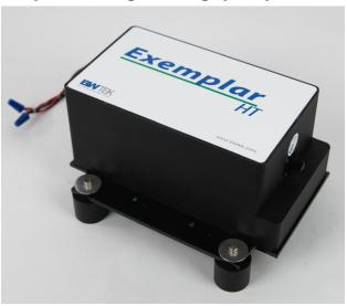
The Exemplar HT (model BTC667N) is a highperformance and high throughput spectrometer which features a low noise deep-cooled (-25°C) back-thinned (BT) CCD detector array with high dynamic range. The unique transmission-optics based spectrograph equipped with the high quantum efficiency detector, provides a superior data quality when configured for use in the 532-1100nm spectral range. The BTC667N offers very high signal-to-noise ratio, making it ideal for ultra low light level applications.
