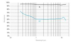
Absorption curves of QS pyroelectric detectors
