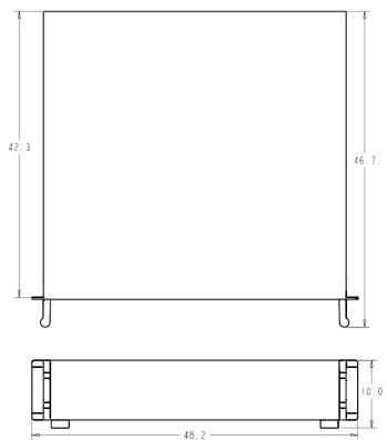
Dimensions of Laser Controller (cm)
