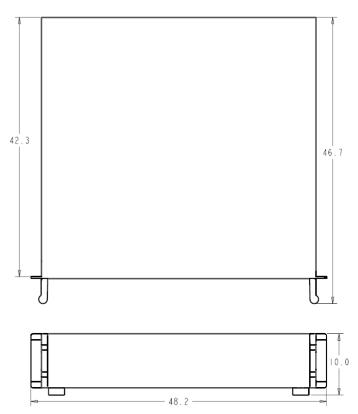
Dimensions of Laser Controller (cm)
