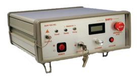
With up to 30 watts of continuous laser power, the BWF2 is a fully integrated turnkey laser solution. The BWF2 combines a high brightness fiber-coupled laser diode, thermoelectric cooler, power supply, and control electronics in a complete package system that operates from a standard wall plug. The BWF2 includes features such as a visible (red) aiming beam, multifunctional relay control for versatile laser operations, remote port for external modulation and control, and an SMA 905 connector.
